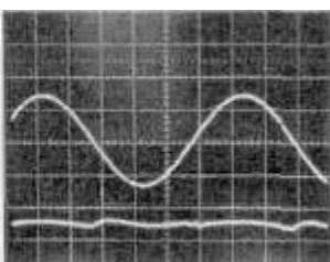
Fig.2: Sine wave 1.6 kHz / 30V RMS / Load = 2 Ohms
