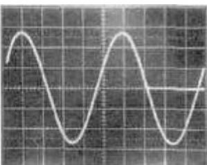
Fig.3: 4:4 Burst 1.6 kHz / 25 V RMS / Load = 1 Ohm
