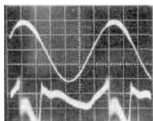
Fig.4: Sine Wave 1.6 kHz / 13V RMS / Load = 8 Ohms
