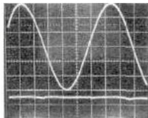
Fig. 1: Sine Wave 1.6 kHz / 40V RMS / Load = 4 Ohms
