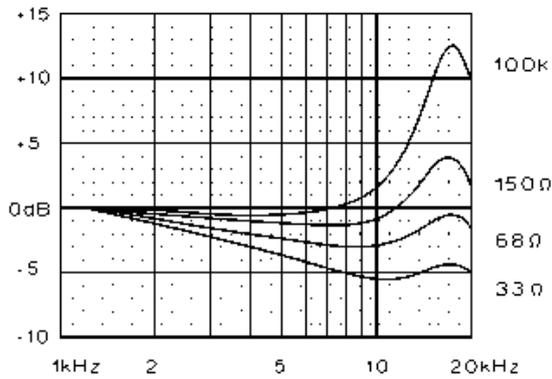
Figure 1 shows the effect of varying the resistive load on a MC cartridge.
