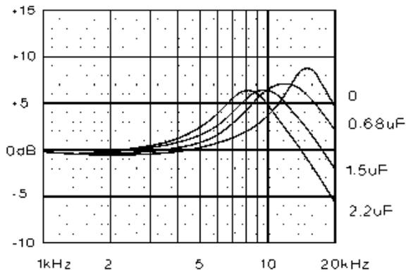
Figure 2 shows the effect of varying the loading capacitance on a MC cartridge.
