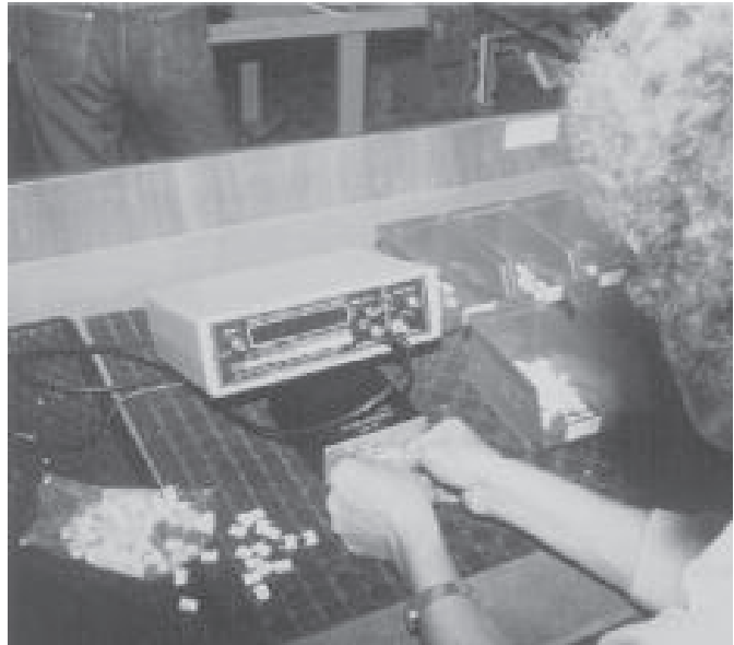
Selecting MIL specified capacitors to even tighter tolerances (to less than 0.1%!); typical tolerances are 10-20%!) to obtained.
