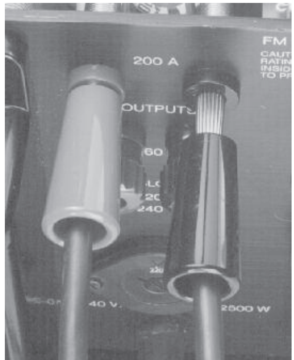
200A output connectors on an FM ACOUSTICS power amplifier. It's details like this that make the difference!
